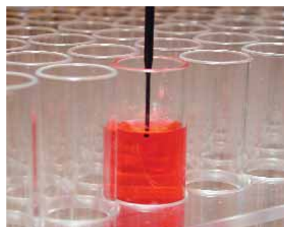
Liquid level sensor with optional clot detection
