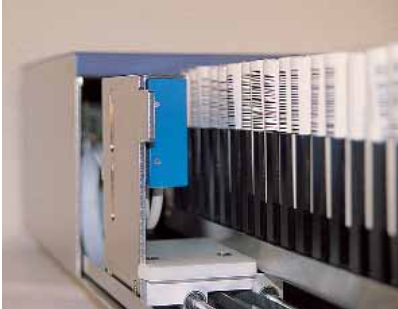
The basic ID-trax module holds 96 samples and can be expanded in batches of 96.
